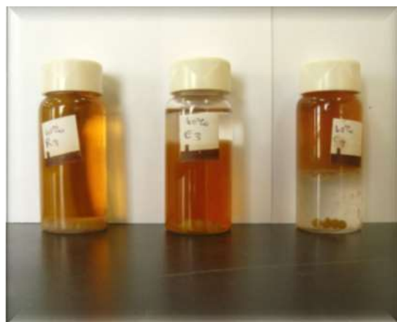
Figure 5. Ethanol, chloroform, and ether extraction of Moringa roots.
