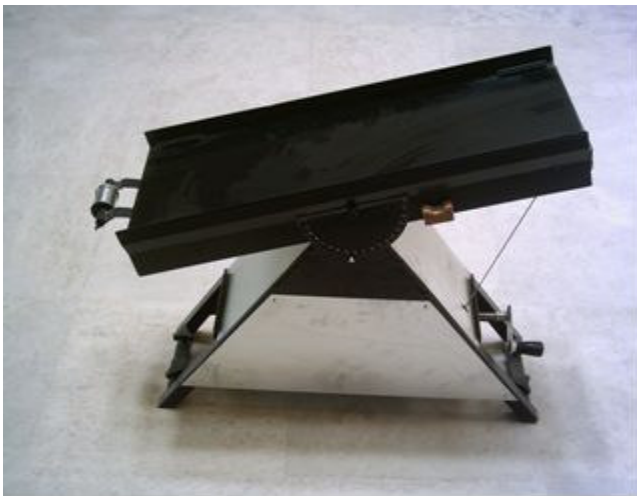
Figure 2. Apparatus to determine coefficient of static friction.
