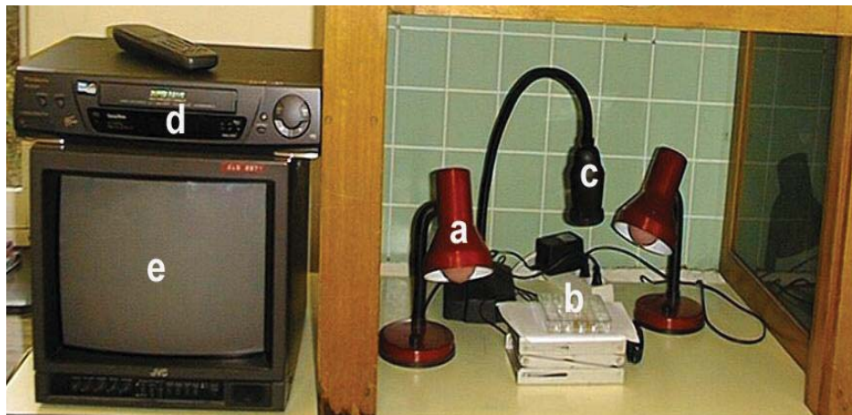
Figure 2. Device use to record the selection of grain hosts by the maize weevil female: (a) red light, (b) box containing insects and grains to be filmed, (c) camera (d) video recorder and (e) monitor.
