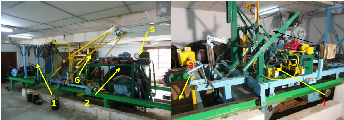
Figure 3. General view of the tire traction testing facility. 1= Drawbar pull loading device, 2= Radial ply tire, 3 = Indoor soil bin, 4 = Soil processing trolley, 5= Dead weight loading platform, 6 = Parallel bar linkage.
