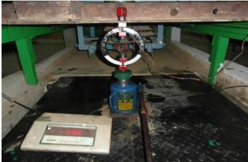
Figure 1. Calibration of ring transducer for measurement of normal load.
