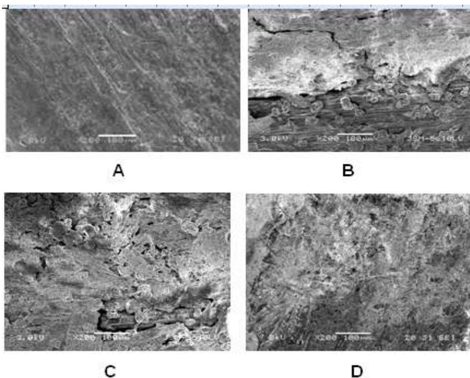
**Figure 1.** Surfaces of plant materials observed by SEM in 15 d. A: the original plant material; B: the plant material treated by B<sub>3</sub> in sterilized; C: the plant material treated by B<sub>3</sub> in non-sterilised soil; D: CK.
