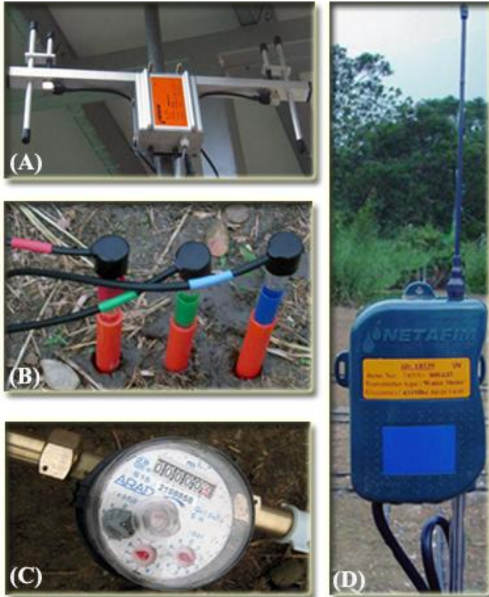
Figure 2. Wireless soil moisture sensory system (Netafim Irrigation Inc.).
