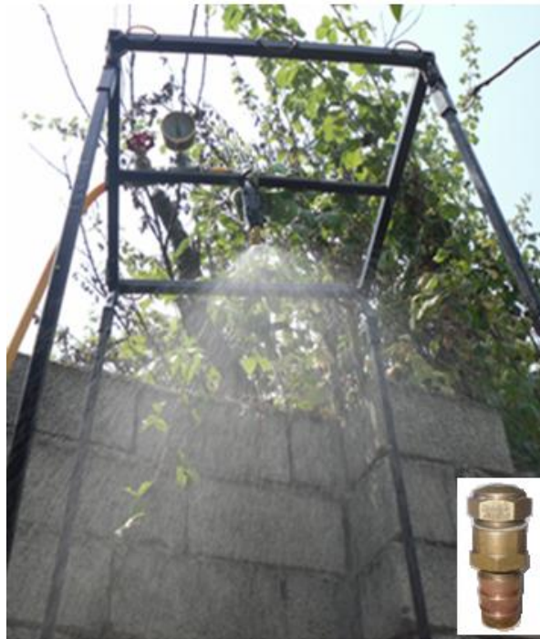
Figure 3. Spraying rain drops from nozzle.
