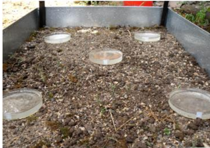
Figure 5. Calibration of the simulator using rain gauges.
