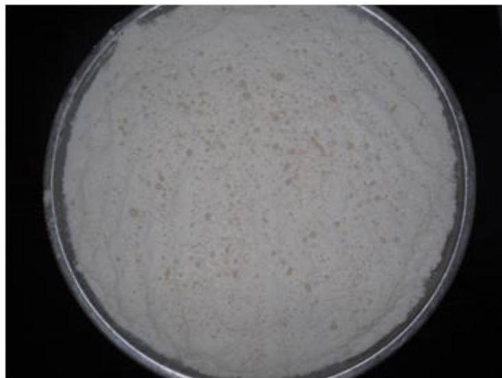
Figure 4. Measuring the diameter of drop impact on flour.
