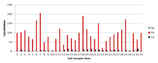
Figure 4. Heavy metal concentrations at each soil sample location close to mechanic workshop.
