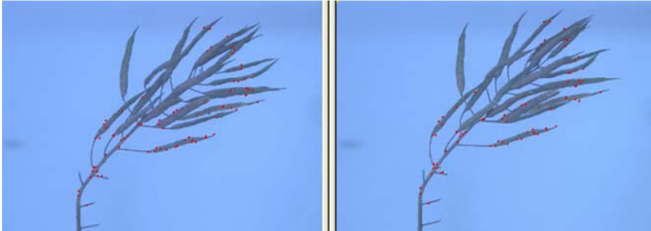
Figure 5. Match results of digital images. Red points represent the matched conjugate points from the two digital images.
