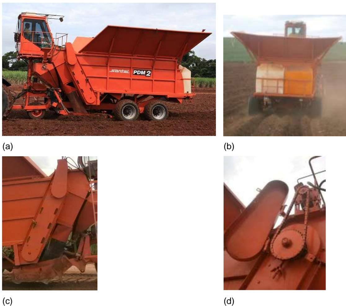
**Figure 1.** Sugarcane billet planter (a and b); billet metering system (c and d).
