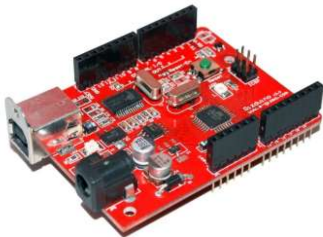
Figure 3. Gizduino 168 development board.
