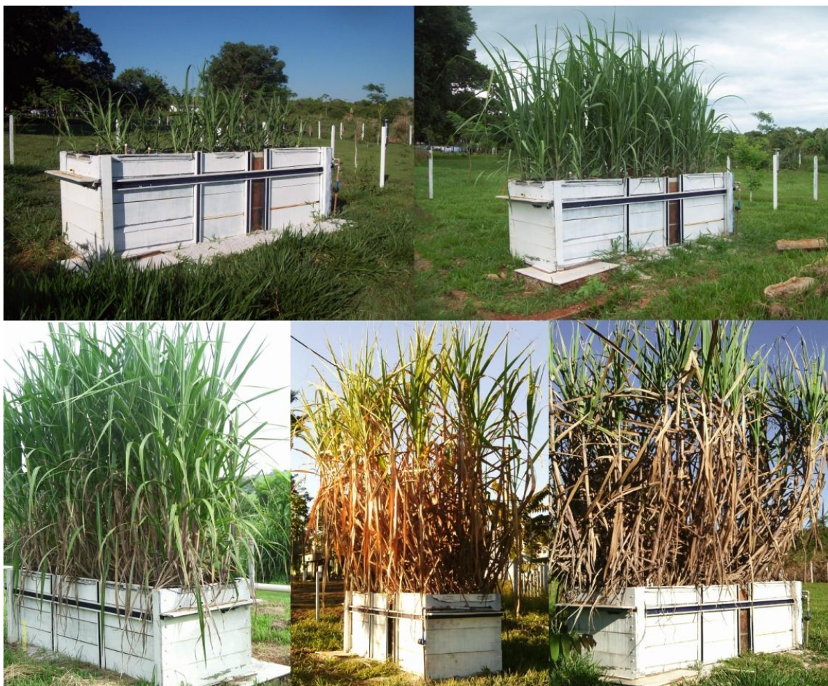
Figure 1. Suspended drainage lysimeter with sugar cane crops at different development phases.
