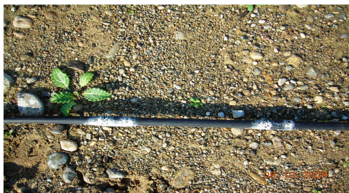
Figure 3. Scale and deposit on laterals during lime-water application.
