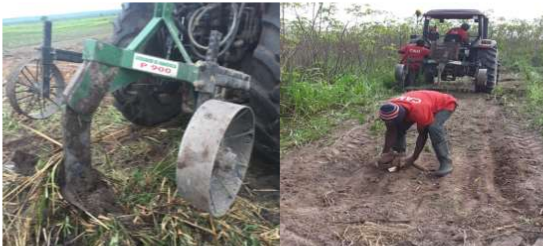
Figure 2. Mechanical harvesting of the roots by plots, at the CAM experimental station, after the vegetative cycle of the crop, with the aid of coupled to the tractor (P900).
