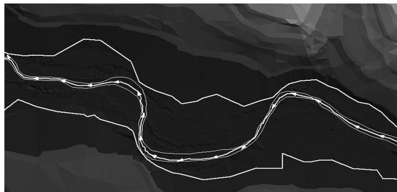
**Figure 4.** Flow path and cross section cut lines themes prepared using the preRAS option in Arc View.
