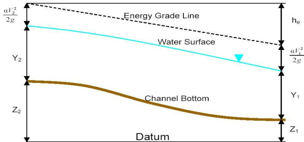
Figure 1. Representation of terms in the energy equation.
