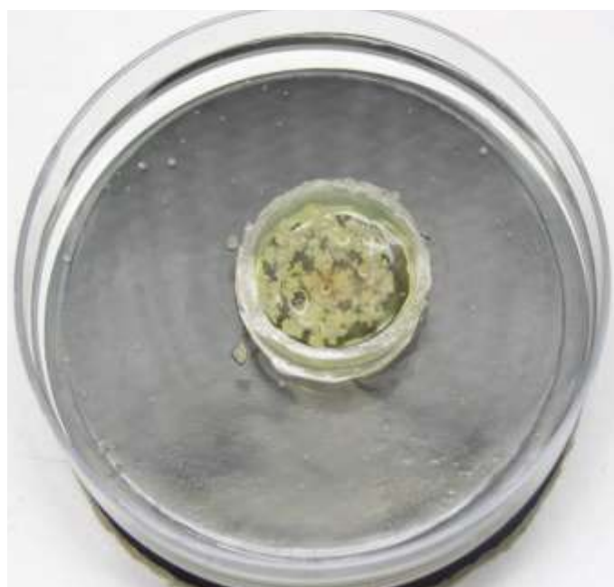
Figure 1. Small sterile plastic ring around the transformed calluses during the detection of \beta -glucuronidase activity.
