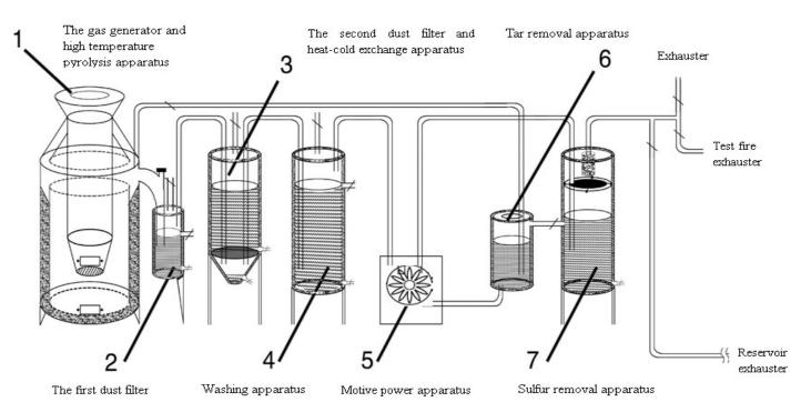
Figure 1. A schematic overview of the whole set-up is shown.
