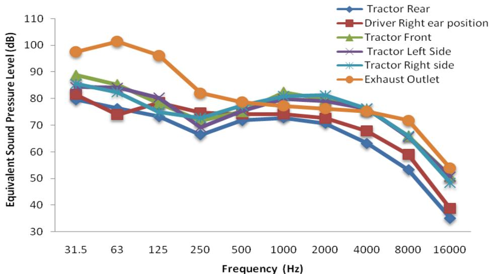
**Figure 3.** Frequency analysis around the MF 285 tractor with idle condition at 1000 rpm.
