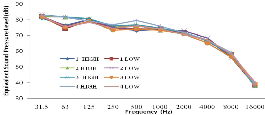
**Figure 6.** Sound level of MF 285 tractor with different gears of gear box and engine speed of 1000 rpm at right ear of driver (L and H stand for low and high gears).
