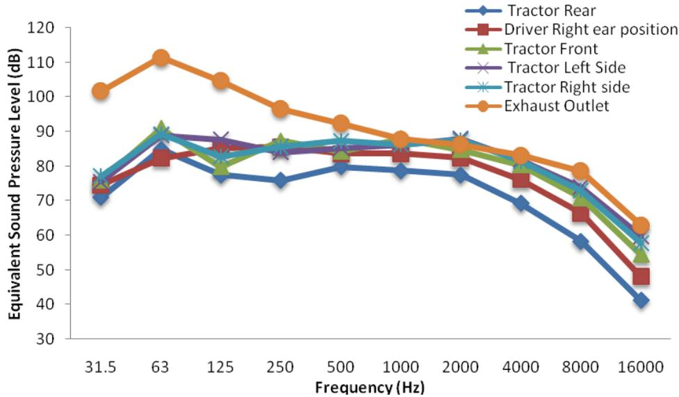
Figure 4. Frequency analysis around the MF 285 tractor with idle condition at 2000 rpm.
