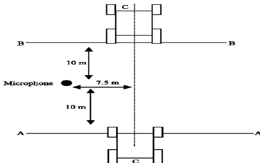
**Figure 1.** Noise level measurements at MF 285 tractor surrounding, derived from Celen and Arin (2003).
