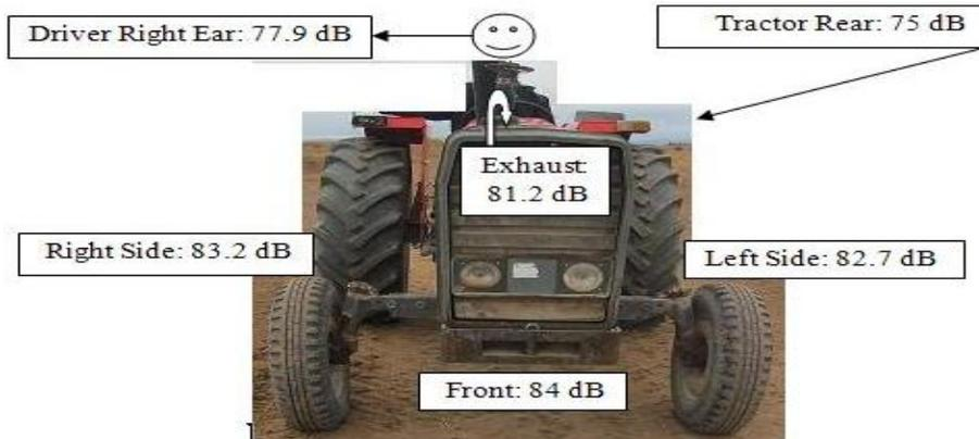
**Figure 2.** The sound pressure level measurements in idle tractor at the surrounding (engine speed was at 700 rpm).
