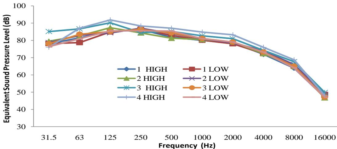
**Figure 7.** Sound level of MF 285 tractor with different gears of gear box and engine speed of 2000 rpm at right ear of driver (L and H stand for low and high gears).
