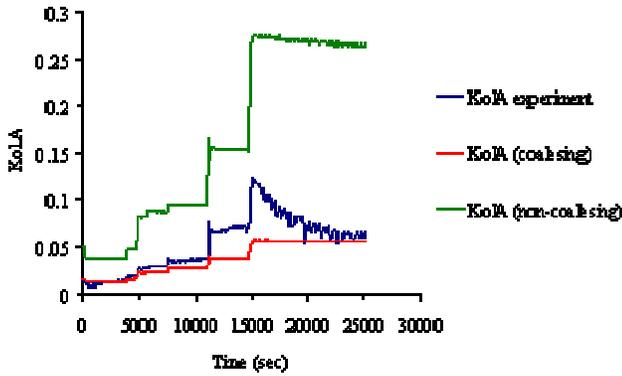
**Figure 7.** Experimental  $K_{ol}A$  compared with coalescing and non-coalescing models.
