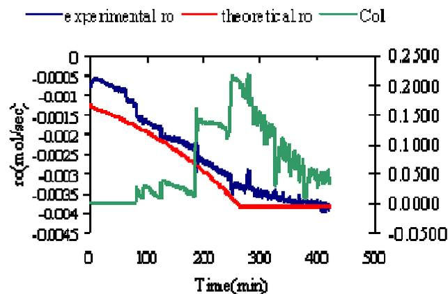
Figure 6. Comparison of theoretical and experimental oxygen production rate versus time.
