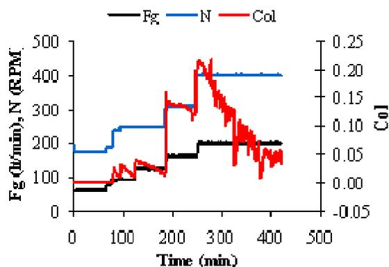
Figure 5. Plot of the concentration of the oxygen in the liquid ( $C_{ol}$ ), stirrer speed ( $N$ ) and gas flow rate ( $F_g$ ) versus time
