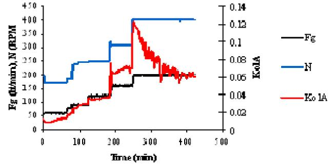
**Figure 8.** The influence of  $F_g$  and  $N$  on the  $K_{ol}A$ .
