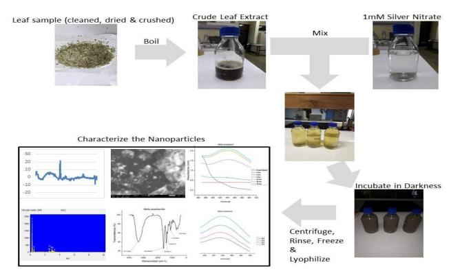
**Figure 1.** The biosynthesis of silver nanoparticles: by mixing the crude leaf extract with silver nitrate, incubating the mixture, centrifuge and lyophilise the AgNPs and then characterise the produced b-AgNPs Source: Authors
