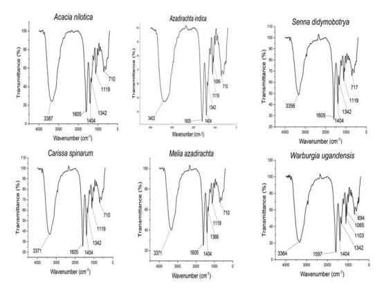
**Figure 4.** The FTIR results indicating the presence and sites (bands) of the biomolecules that are responsible for reducing the AgNO<sup>3</sup> to b-AgNPs as well as those responsible for capping and stabilising the AgNPs Source: Authors
