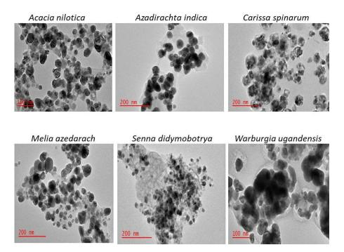
**Figure 5.** The TEM results indicating the sizes and shapes of the b-AgNPs that were produced using crude extracts from the different medicinal plants. Source: Authors
