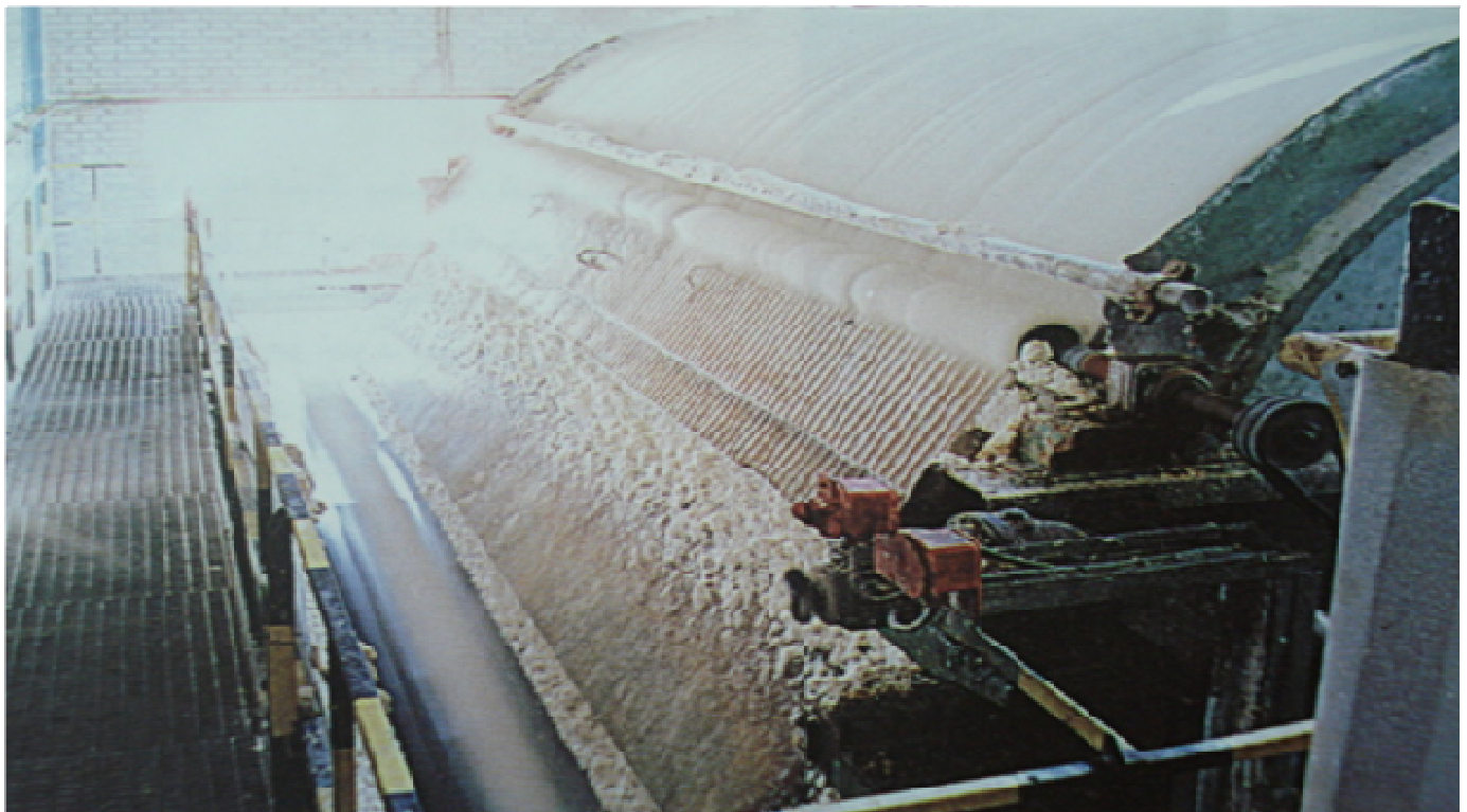
Figure 3. Pulp screening and cleaning in Pars Paper Factory.
