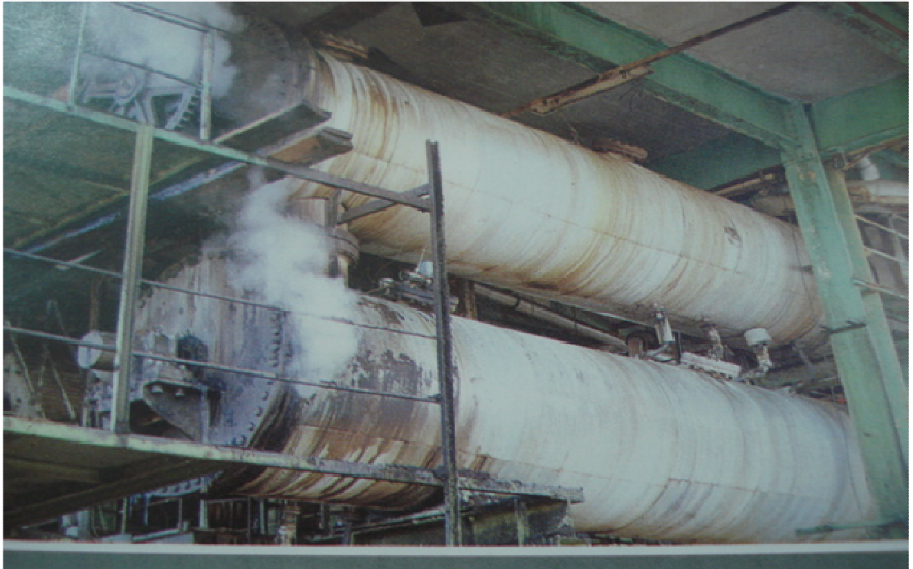
Figure 2. Cooking process on pulp mill in Pars Paper Factory.
