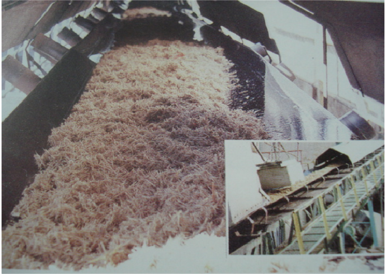
Figure 1. Transported bagasse through the conveyer belts from the sugarcane factory to the paper factory.
