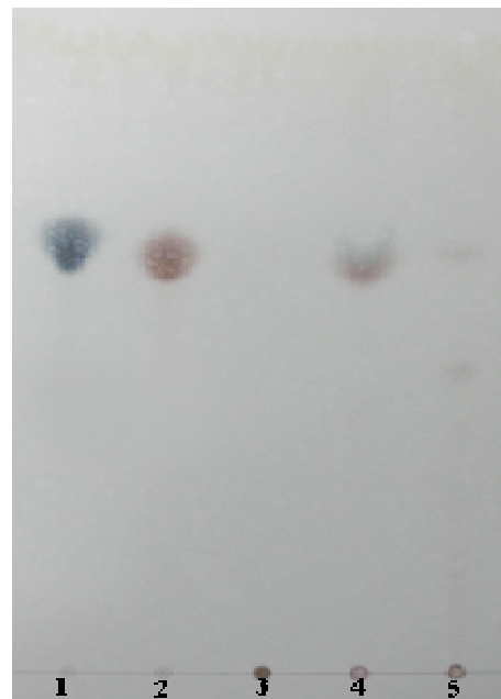
Figure 2. TLC chromatogram of hydrolysis products of inulin by inulinolytic enzymes from M. koreense LS-A18 and N. lucentensis MH-F19. Lane 1 glucose, Lane 2 fructose, Lane 3 inulin (Sigma); Lane 4 hydrolysis products by inulinase from strain LS-A18; Lane 5 hydrolysis products by inulinase from strain MH-F19. Volume of samples 3 \mu l.
