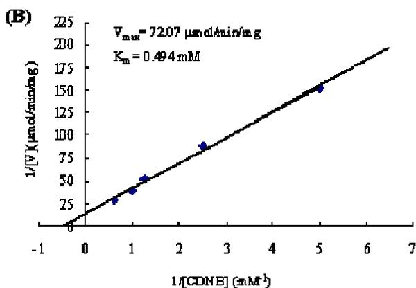
**Figure 2.** Lineweaver-Burk plot of enzyme activity of the purified *BmGST* with varying concentrations of (A) glutathione (0.2-2.4 mM) or (B) CDNB (0.1-1.6 mM) at a fixed concentration of CDNB (1 mM) or glutathione (5 mM), respectively. Values are means based on at least 3 replicates.
