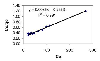
Figure 6. The linearized Langmuir adsorption isotherm of direct dye by fungal biomass at pH 5.5 and T =  $28-30^{\circ}$ C.
