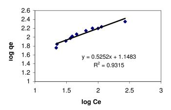
**Figure 8.** The linearized Freundlich adsorption isotherm of direct dye by fungal biomass at pH 5.5 and  $T = 28 - 30^{\circ}C$ .
