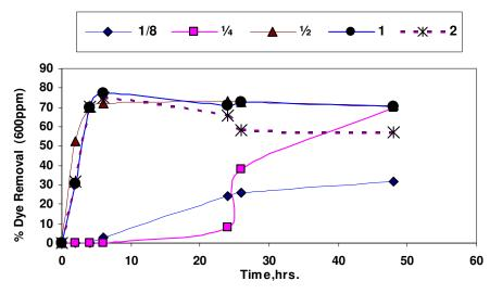
Figure 2. Effect of aeration on removing of dis-azo dye using fungal strain 20 (after addition 600 ppm dye).
