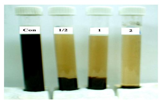
Figure 1. Removal of direct brown dye by A. niger strain at ½, 1, 2 v/v/min. aeration rate after 10 h incubation.
