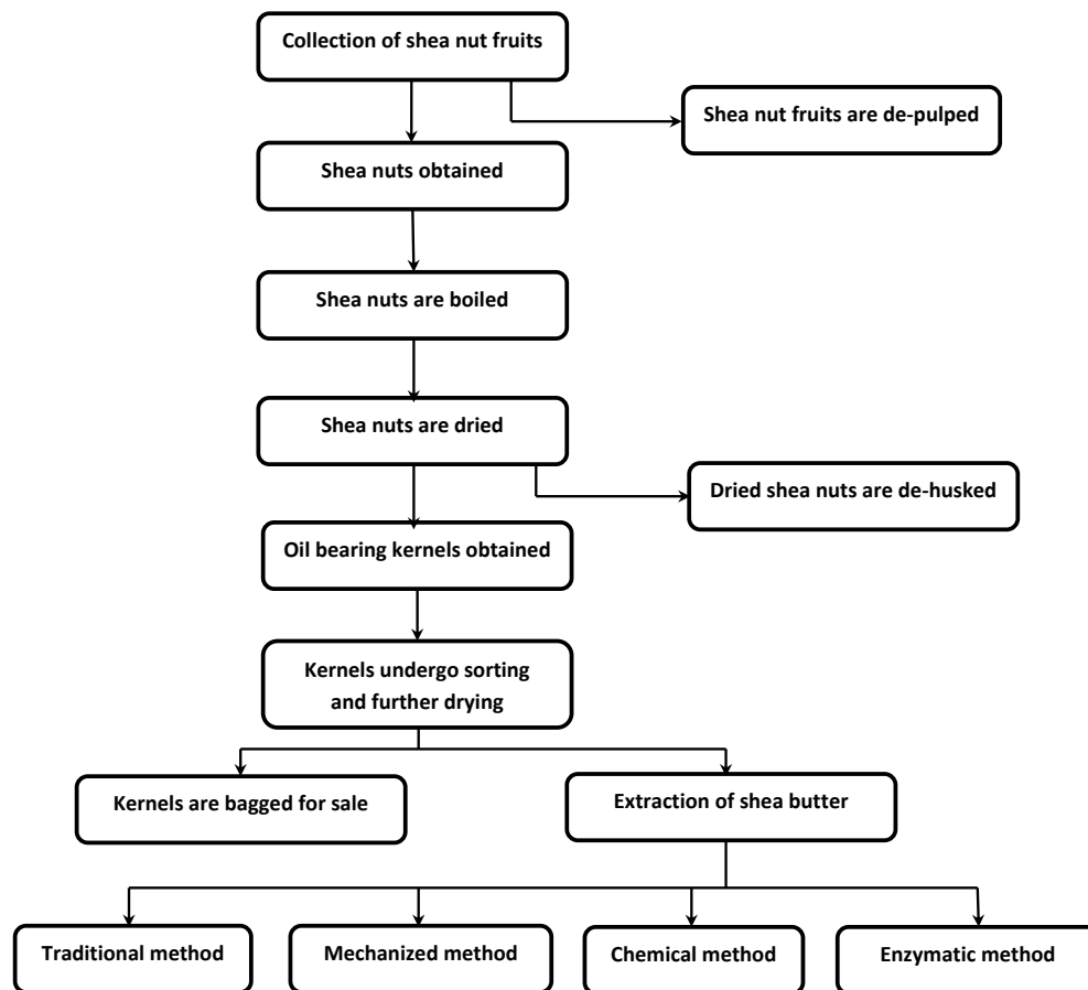
Figure 3. General pre–treatment of the shea nut fruit to obtain the kernel (Abdul–Mumeen, 2013; Moore, 2008 descriptions).
