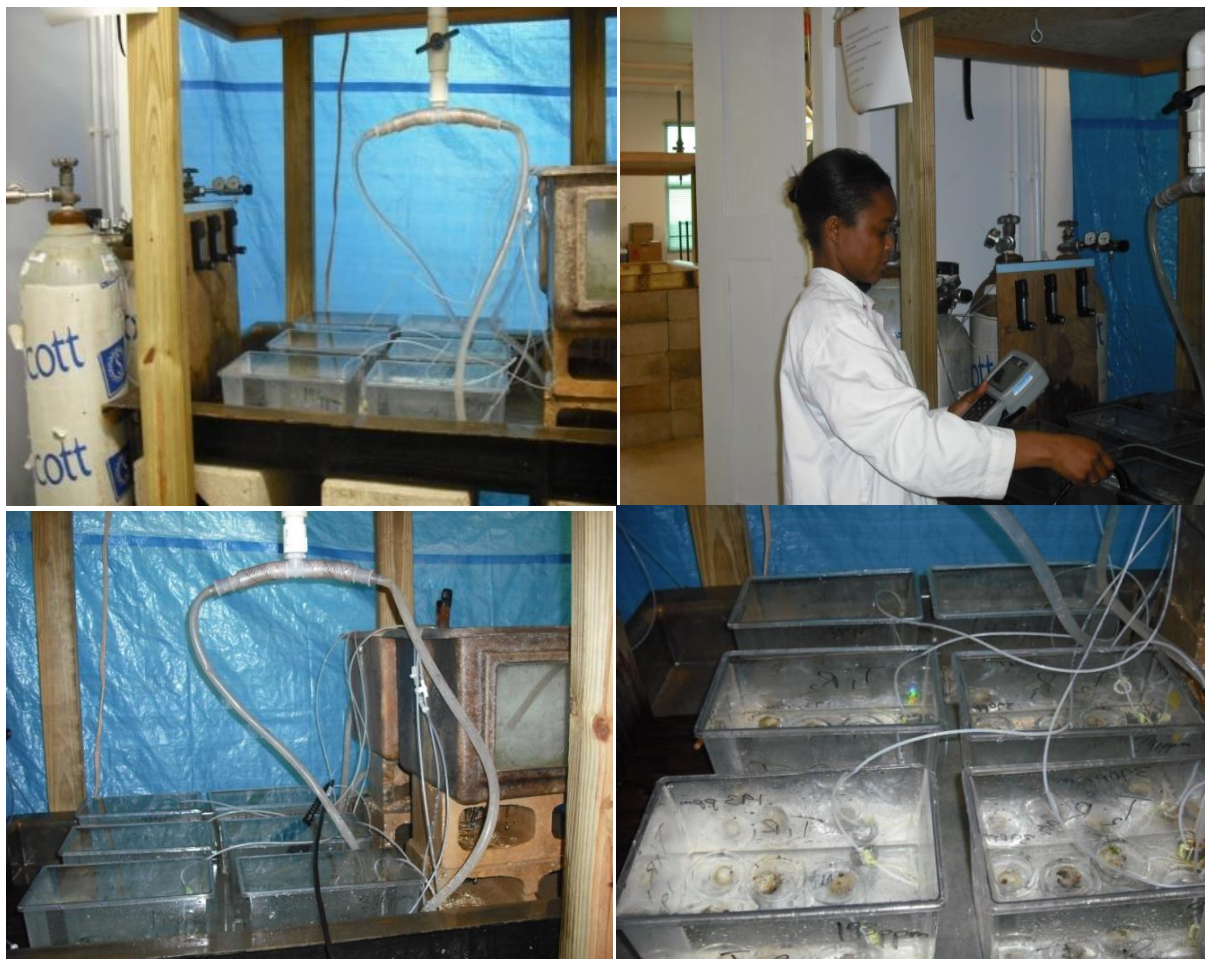
Figure 2. A set up of manipulated CO 2 acidified seawater flow-through system at Bermuda Institute of Ocean Science. The experimental tanks (control tanks, n = 3 and acidification tanks, n = 3). Physicochemical parameters in the experimental tanks were measured using YSI 556 Multiple Parameter Handheld Sonde.
