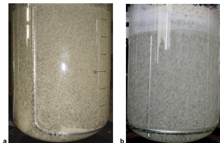
Figure 4. The morphology of LA-UN-1 in bioreactor (a) and after the 10th run of the repeated batch culture (b).
