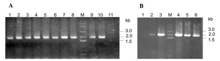
Figure 3. Agarose gel (0.8%) electrophoresis analysis of PCR products generated with *cry8D*-specific primers. (A) Lanes 1–8: strains MSS1.2, MSS1.3, MSS1.4, MSS2.3, MSS2.4, MSS2.7, MHY1.1, MHY1.3; lane M: Marker (10,000 bp); lane 9: MHY1.10; lane 10: MHY3.8; lane 11: Negative control (Btk). (B) Lane 1: Negative control (Btk); lane 2: MHB10.6; lane 3: MHB11.5; lane M: Marker (10,000 bp); lanes 4-6: MHB11.3, MHB9.3, MHB5.2.
