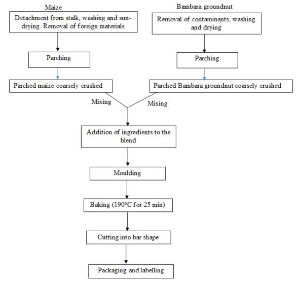
Figure 2. Flow chart for the production of snack bar.
