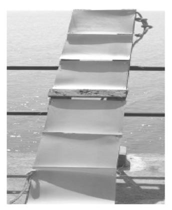
Figure 1. The Biofilm development rack.
