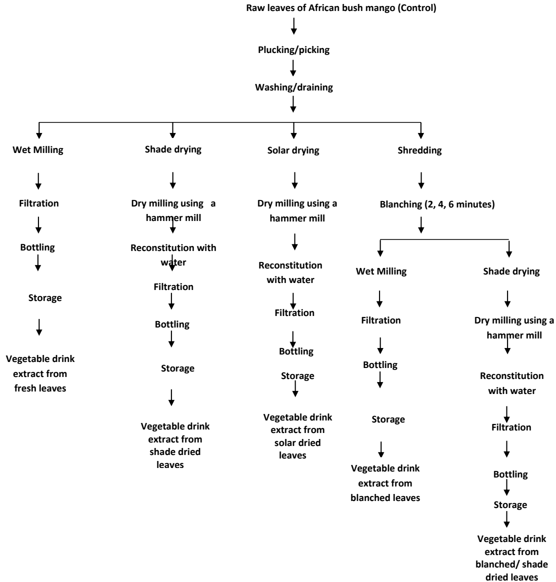
Figure 1. Flow diagram for the preparation of vegetable drink extract from from raw (control treatment), raw/dried, blanched (2, 4 and 6 min), blanched/shade-dried (2, 4 and 6 min), leaves of Irvingia gabonensis .
