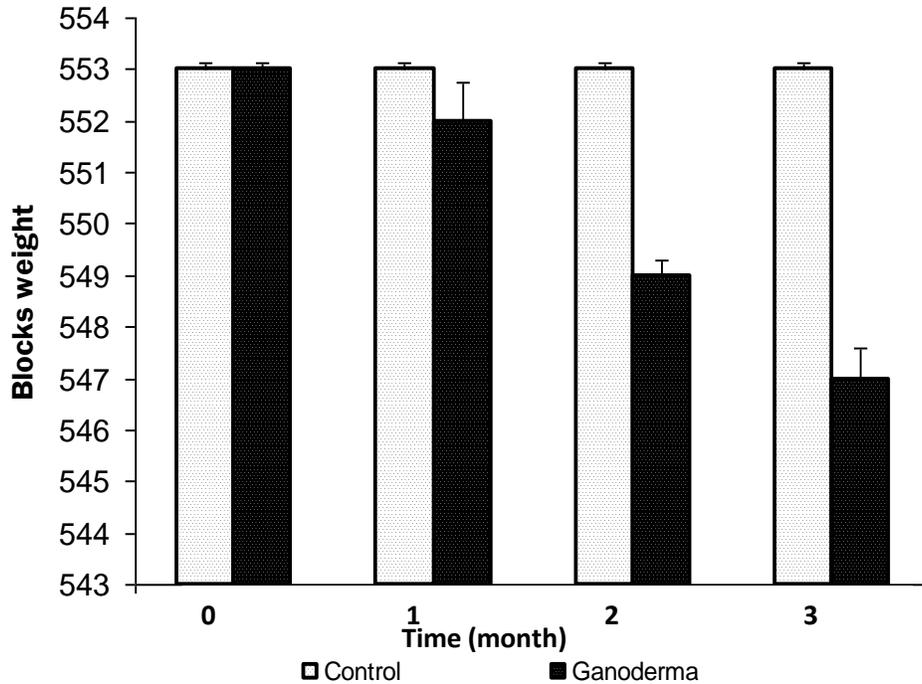
**Figure 1.** Wood decay test of *Ganoderma boninense* (the test was carried out over three months).
