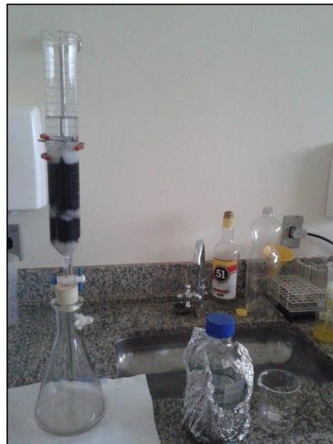
**Figure 2.** Charcoal column used for filtration of the cachaça obtained from fermented must produced with the selected and compressed yeast.
