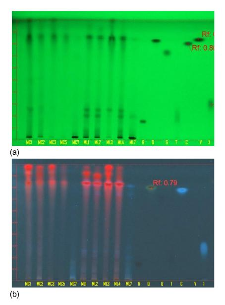
**Figure 2.** Chromatograms of extracts sample and standard in HPTLC analysis (a) under UV 254 nm, (b) under 366 nm. *M. charantia* (MC1, ethanol; MC2, methanol; MC3, ethyl acetate; MC6, Chloroforme; MC7, water); *M. lucida* (ML1, ethanol; ML2, methanol; ML3, ethyl acetate; ML4, acetone; ML7, water); Standards (R, Rutin; Q, Quercetin; G, acid Galic; T, acid Tanic; C, acid cafeic; V, acid Vanilic; Cl, acid Clorogenic).
