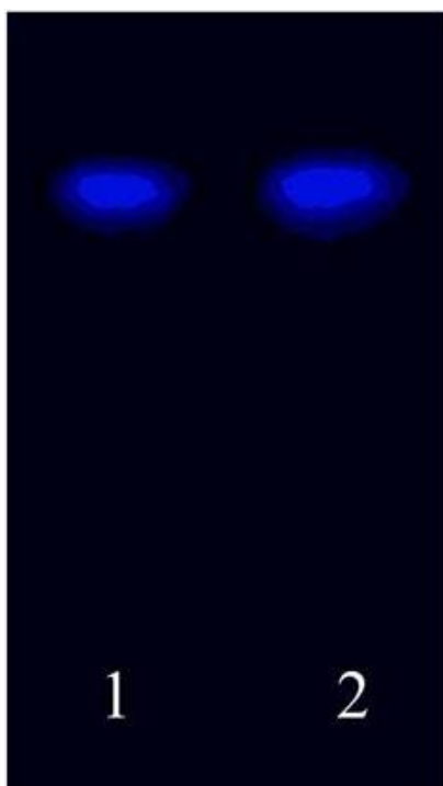
Figure 2. Chromatography of AFB 1 spot in the presence of chloroform extract. Lane 1, Standard AFB 1 , lane 2, AFB 1 sample extracted from A. Flavus . TLC was run in the solvent system of chloroform:acetone (85:15).
