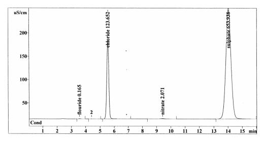
Figure 4. Chromatogram of common anions in drinking water sample for Wathba plant.
