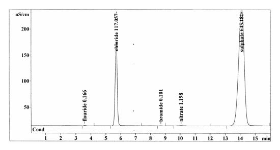
Figure 3. Chromatogram of common anions in raw water sample for Wathba plant.
