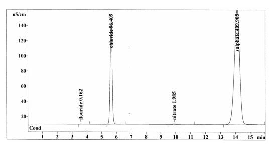
Figure 2. Chromatogram of common anions in drinking water sample for east Tigris plant.
