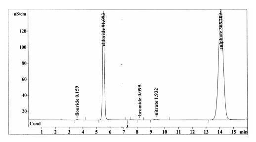
Figure 1. Chromatogram of common anions in raw water sample for East Tigris Plant.
