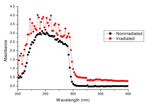
Figure 2. Variation in the absorbance values of the irradiated and nonirradiated films (60 phr).
