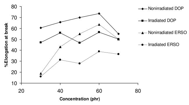
Figure 4. Variation in elongation at break with plasticizer concentration.
