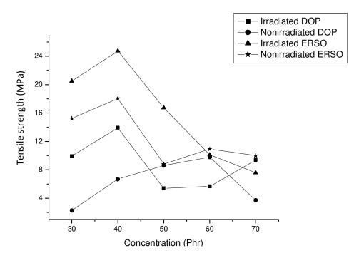
Figure 3. Variation in tensile strength with increase in plasticizer concentration.
