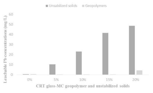
**Figure 3.** Concentration of extractable lead in unstabilised starting materials and CRT glass-MC geopolymer counterparts.
