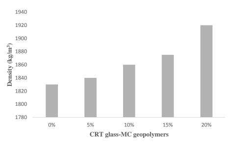
Figure 2. Dry density of CRT glass-metakaolin geopolymers at 28 days.
