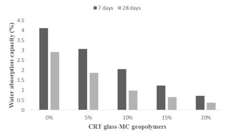
Figure 1. % Water absorption capacity of CRT glass-MC geopolymers at 7 and 28 days.
