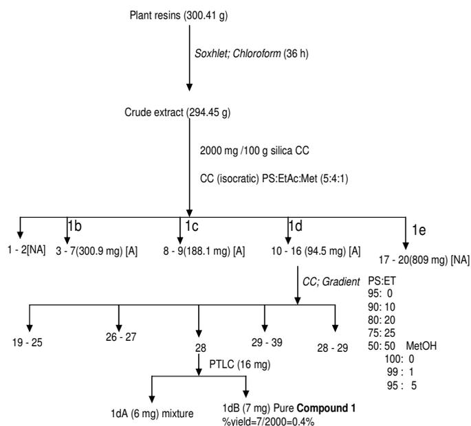
**Figure 2.** Scheme of isolation of active principles from resin of *C. glandulosa* extract. PS, petroleum spirit; ET, ethylacetate; MetOH, methanol; CC, Column chromatography; TLC, preparative TLC; [A], active (inhibition of microbial growth); [NA], not active (lack of inhibition of microbial growth).
