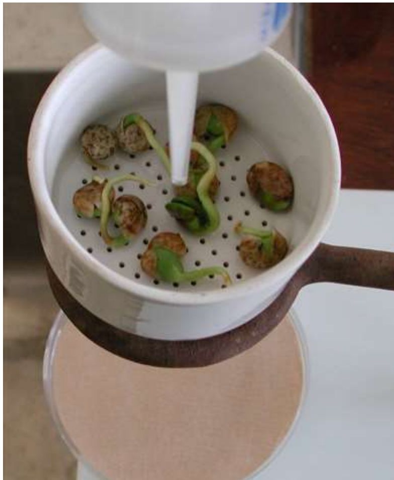
Figure 2. Illustration of the set-up for funnelling leachates from a Büchner funnel to a Petri-dish for germination studies on the effects of leachates from seedlings of selected rotational crops and ryegrass.
