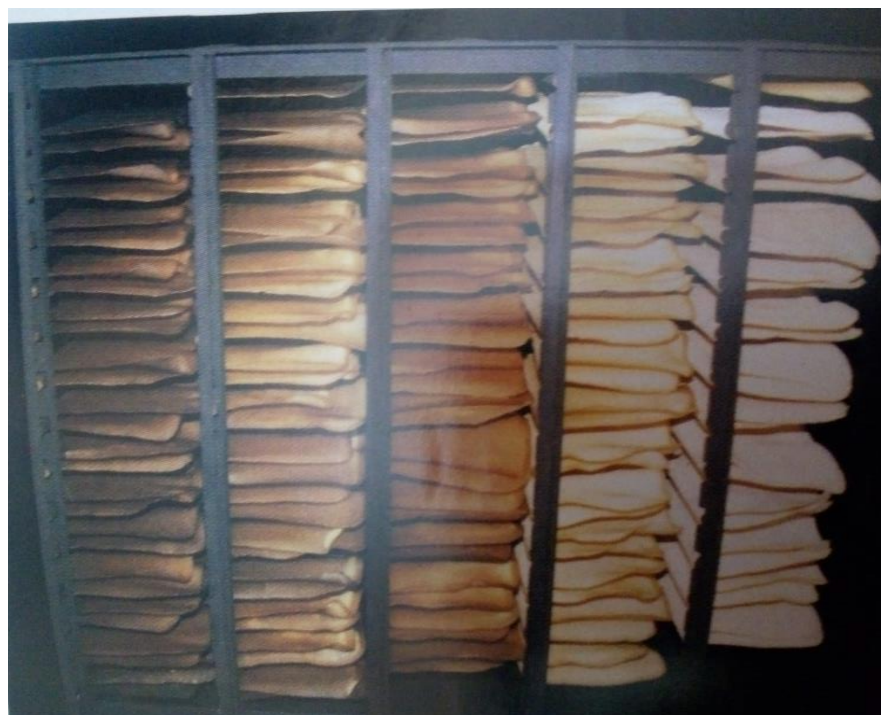
Figure 2. Rubber sheets hung on reapers in a smokehouse. Source: Aigbodion (2017).
