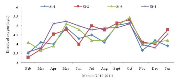
Figure 8. Variations in dissolved oxygen (mg/l) recorded at four different stations.
