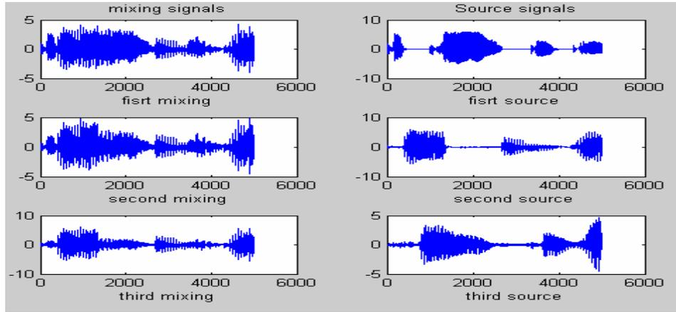
Figure 2. The mixing signals in left and original signals in right.
