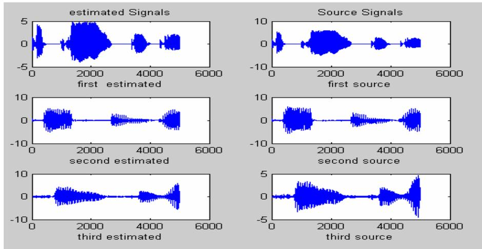
Figure 3. The estimated signals in left with scales, permutation and original signals in right.
