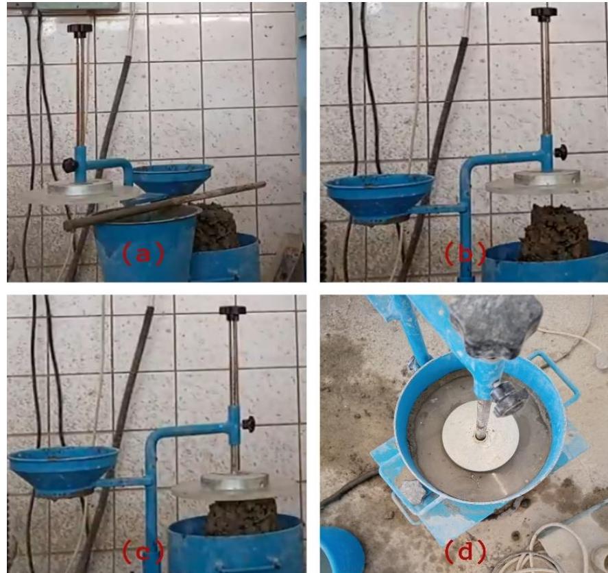
Figure 3. (a) Vebe slump (b) Glass disk raised to 0cm height (c) Depth of first drop of Vebe rod (d) Mortar ring appears on the sides of the transparent glass disk.
