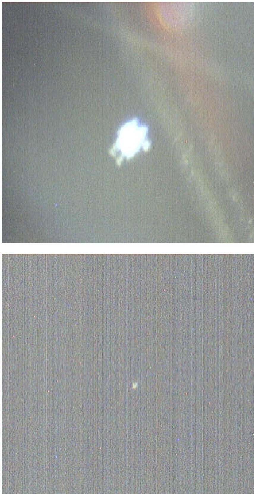
Figure 3. CCD Images of a bubble captured with the continuous Xe lamp (upper) or a single-shot of the Xe flashlamp (lower). The image width spans the actual scale of 3.27 mm.
