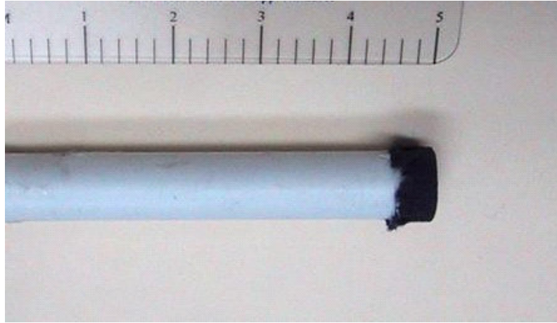
Figure 1. RH sensor packaged for embedding in concrete.
