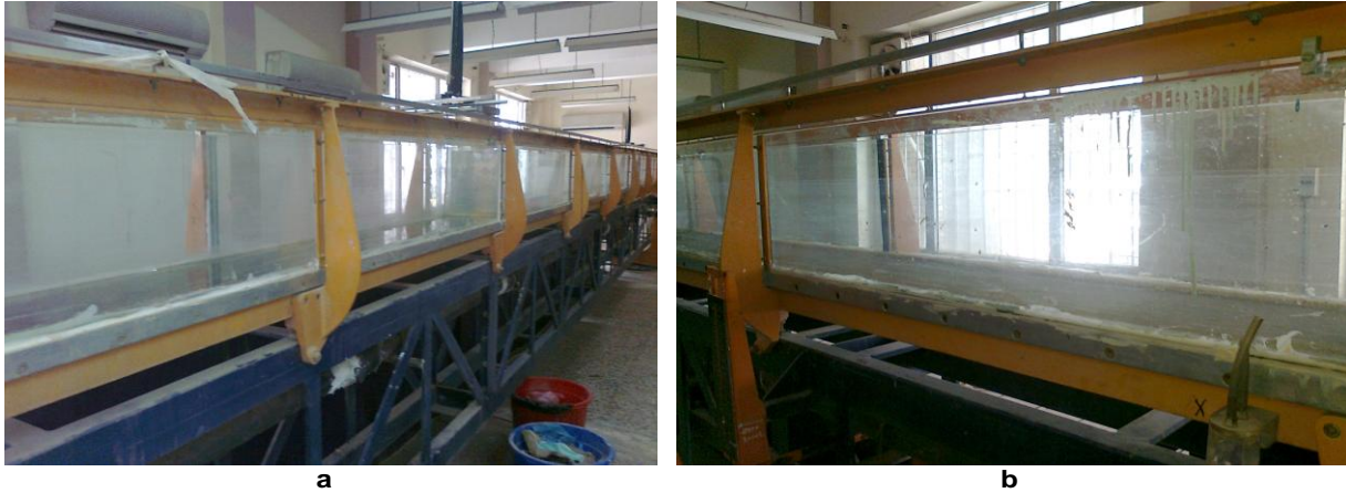
Figure 1. Open channel used in the experiments.
