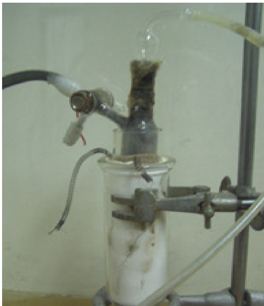
Figure 4. Hydrogen storage micromeritics apparatus with carbon fiber and Trinaphthalenohexahydro[12] annulene.
