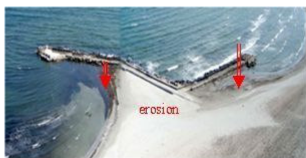
Photo 4. Local effects of erosion on the backshore - groin in southern part of Mamaia bay (17 III 2003).
