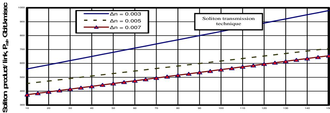
Figure 14. Variations of the soliton product/link with fiber cable length at the assumed set of parameters. Fiber cable length, L, km.
