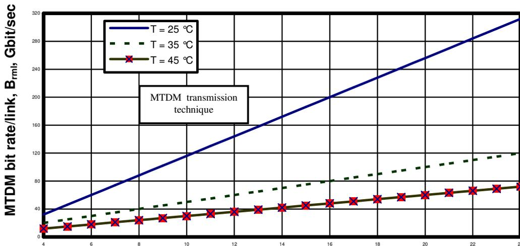
**Figure 19.** Variations of the MTDM bit rate/link with number of links in fiber cable at assumed set of parameters. Number of links in the fiber cable core,  $N_L$ .
