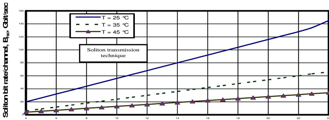
Figure 16. Variations of the soliton bit rate/channel with number of links in fiber cable at assumed set of parameters. Number of links in the fiber cable core,  $N_L$ .
