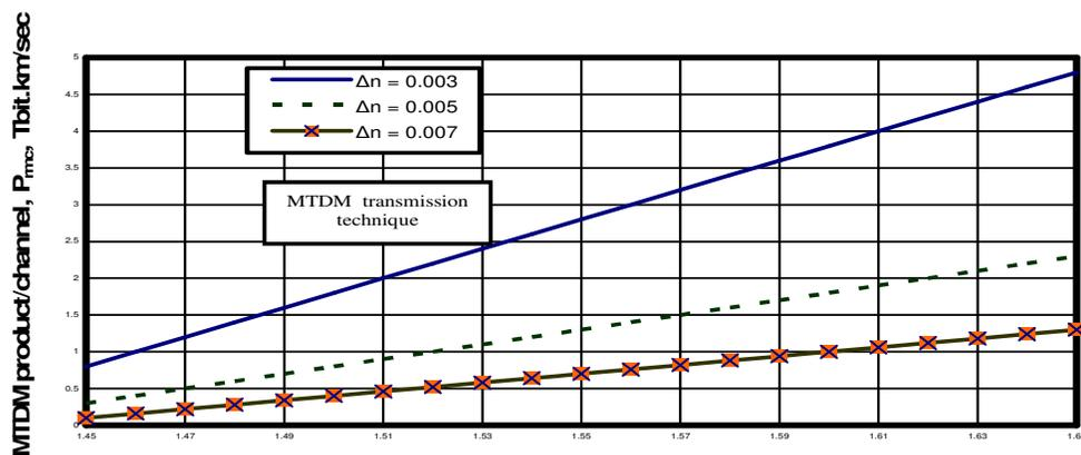
Figure 9. Variations of the MTDM product/channel with optical signal wavelength at the assumed set of parameters. Optical signal wavelength,  $\lambda$ ,  $\mu\text{m}$ .
