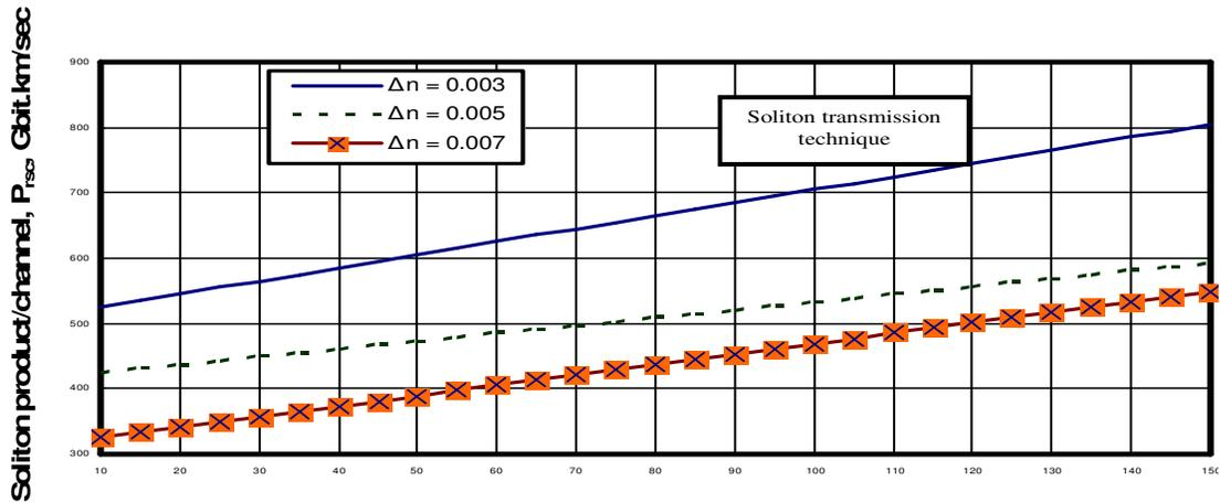
Figure 12. Variations of the soliton product/channel with fiber cable length at the assumed set of parameters. Fiber cable length, L, km.
