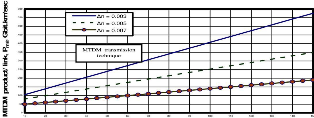
Figure 15. Variations of the MTDM product/link with fiber cable length at the assumed set of parameters. Fiber cable length,  $L$ , km.
