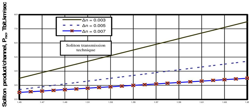
Figure 8. Variations of the soliton product/channel with optical signal wavelength at assumed set of parameters. Optical signal wavelength,  $\lambda$ ,  $\mu\text{m}$ .
