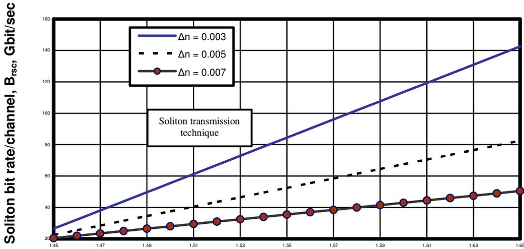
Figure 2. Variations of the soliton bit rate/channel with optical signal wavelength at the assumed set of parameters. Optical signal wavelength,  $\lambda$ ,  $\mu\text{m}$
