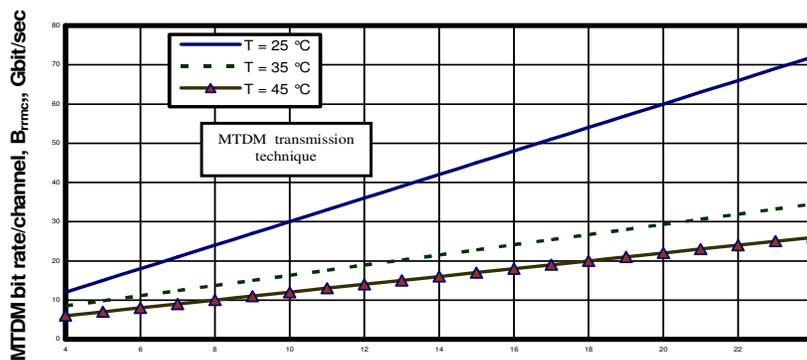
Figure 17. Variations of the MTDM bit rate/channel with number of links in fiber cable at assumed set of parameters. Number of links in the fiber cable core,  $N_L$ .
