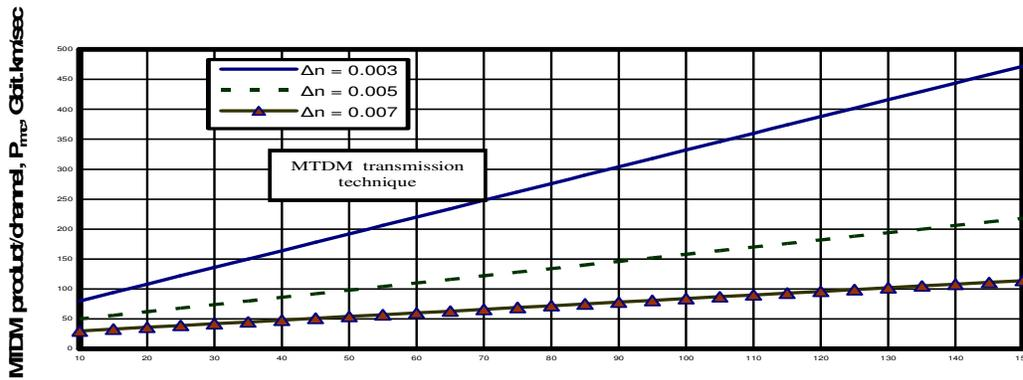
Figure 13. Variations of the MTDM product/channel with fiber cable length at the assumed set of parameters. Fiber cable length, L, km.
