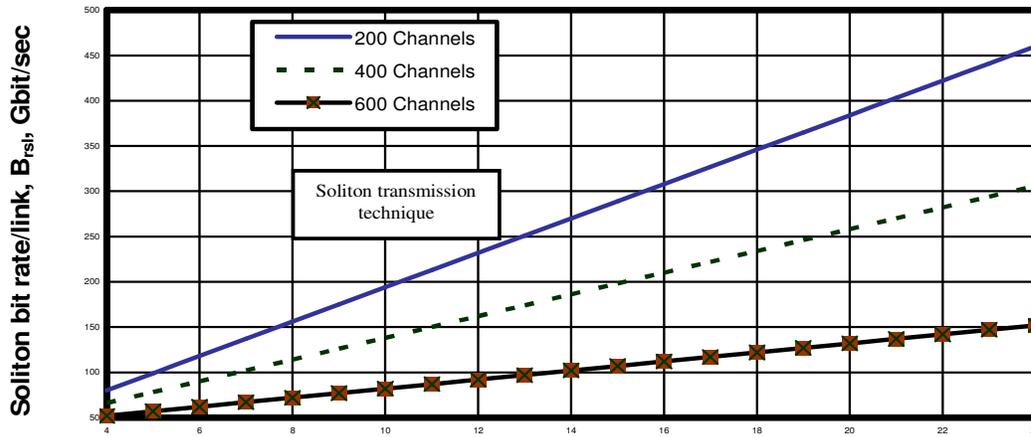
Figure 4. Variations of the soliton bit rate/link with number of links in fiber cable at assumed set of parameters. Number of links in the fiber cable core,  $N_L$ .
