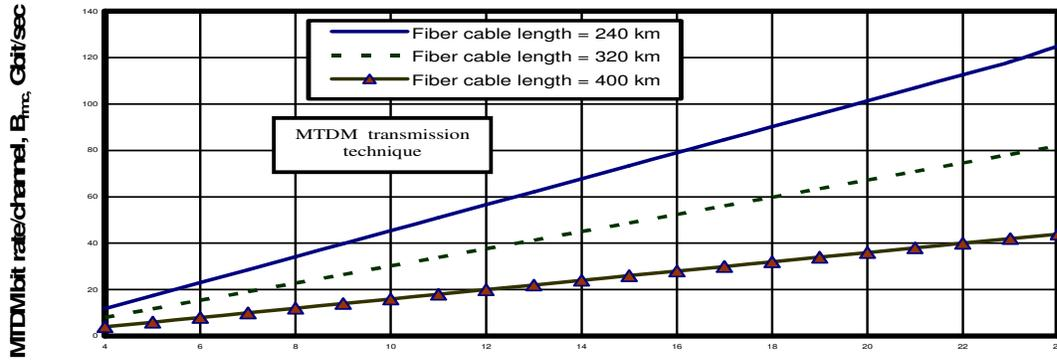
Figure 7. Variations of the MTDM bit rate/channel with number of links in fiber cable at assumed set of parameters. Number of links in the fiber cable core,  $N_L$ .
