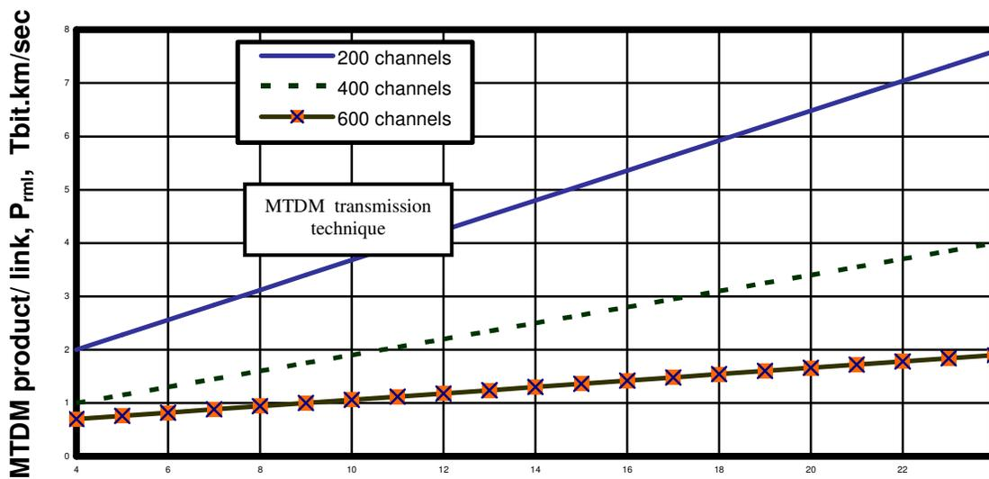
Figure 11. Variations of the MTDM product/link with number of links in fiber cable at assumed set of parameters. Number of links in the fiber cable core,  $N_L$ .
