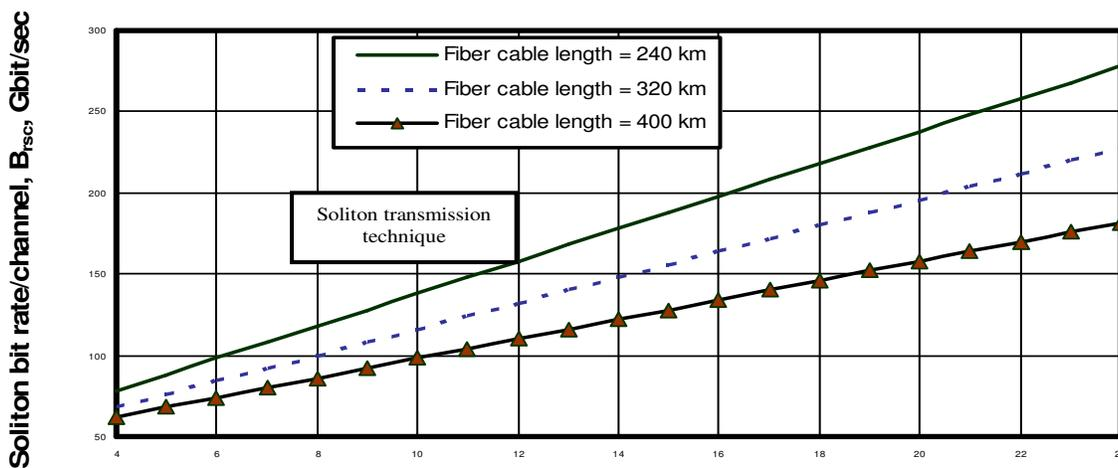
Figure 6. Variations of the soliton bit rate/channel with number of links in fiber cable at assumed set of parameters. Number of links in the fiber cable core,  $N_L$ .
