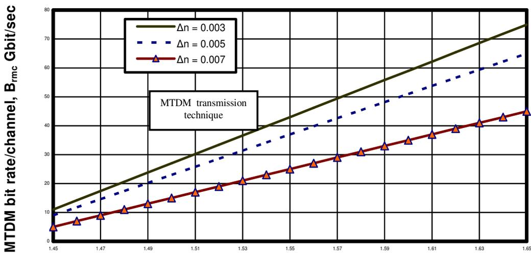
Figure 3. Variations of the MTDM bit rate/channel with optical signal wavelength at the assumed set of parameters. Optical signal wavelength,  $\lambda$ ,  $\mu\text{m}$ .
