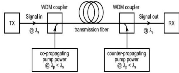
**Figure 1.** Schematic of a distributed Raman fiber amplifier. The pump power at wavelength  $\lambda_p$ , often provided by Raman fiber lasers, may be co- or counter-propagating (or both) with the signal to be amplified at  $\lambda_s$ .
