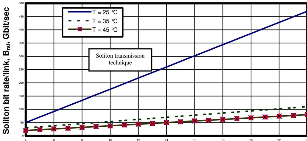
**Figure 18.** Variations of the soliton bit rate/link with number of links in fiber cable at assumed set of parameters. Number of links in the fiber cable core,  $N_L$ .
