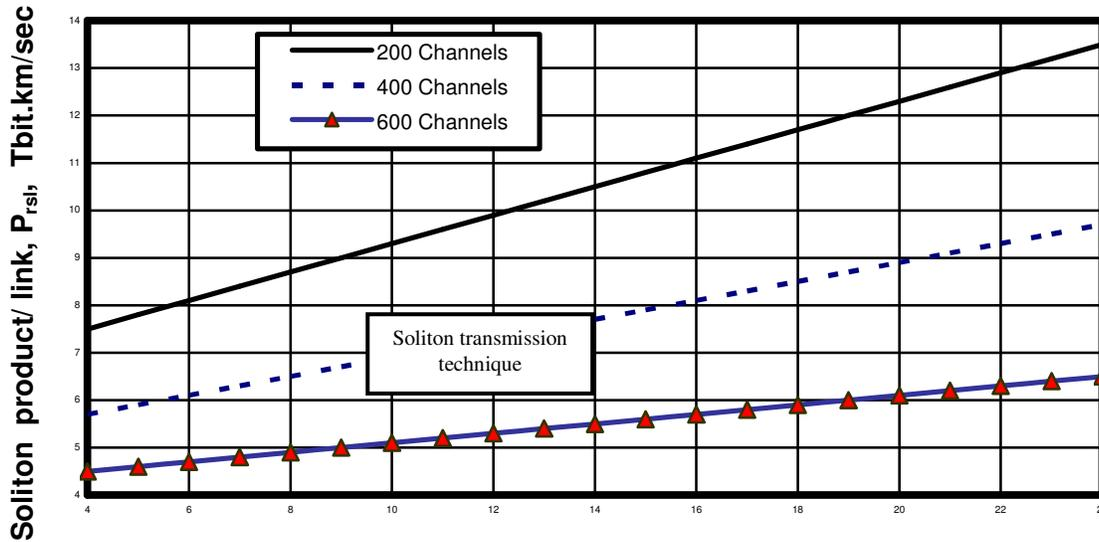
Figure 10. Variations of the soliton product/link with number of links in fiber cable at assumed set of parameters. Number of links in the fiber cable core,  $N_L$ .
